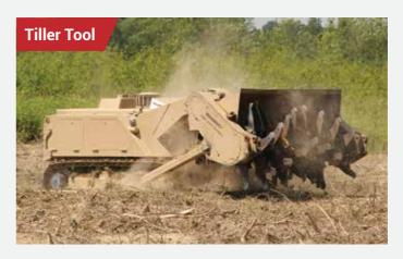
The MV-4 tiller head is another solution for both mine clearance and mechanical ground preparation operations. Its stiff levers with claws made of special steel are highly resistant to detonations, tier and wear.
