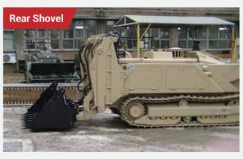
This is another rear exchangeable tool for logistic support operations. It can be used in a limited-scale construction activities.
