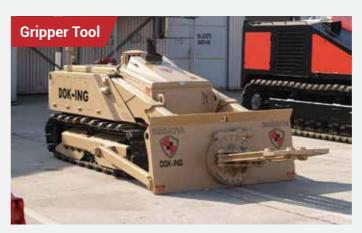
The rotational Gripper is used primarily as rescue and cutting tool, to remove road blocks and other obstacles, safely handle dangerous objects with the maximum lifting capacity of 1500 kg.
