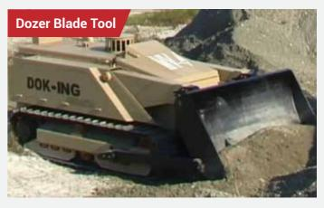
The Dozer Blade enables the MV 4 to work in soil containing ERW, to remove debris, road blocks and other obstacles, and to conduct limited-scale fortification activities.
