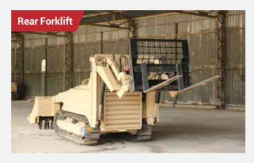
This is the rear exchangeable tool primarily used in support operations: to lift various objects with the maximum loading capacity up to 800 kg, and can also be used as a "mule".
