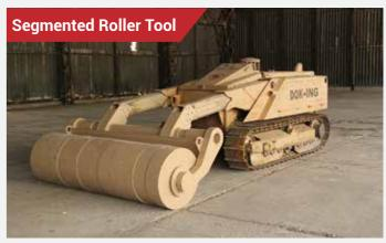
The Segmented Roller is another exchangeable tool primarily suitable for a limited-scale mine clearance of paths and small roads, area proofing, providing less disturbance to soil. It operates by pressure and rotation of its 12 independent rollers. The Segmented Roller is useful for verification of already cleared ground as well as a confidence building tool among local population.
