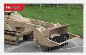
The MV-4 with a standard flail head is a versatile remotely operated system that can be utilized in a number of scenarios: as the Mine Clearance Machine (MCM) to detonate hazards or as the Mechanical Ground Preparation Equipment (MGPE) to improve efficiency of mine clearance operations by reducing or removing obstacles: vegetation cutting and clearing, removal of tripwires, loosening of soil, removal of metal contamination, debris, boulders, rubble, others.
