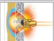
As the bullet hits the plate, the hard ceramic strike face begins to break up the bullet while the ballistic material begins to absorb the energy of the penetration.
