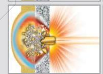
The round continues to break apart as the ballistic material extracts energy, decelerating the projectile and catching the fragments while limiting the effect of blunt trauma, the injury caused by an impacting bullet.
