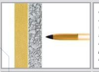
Ceramic plates are designed to stop rifle rounds and armor-piercing rounds which have a penetrating steel pin in the bullet. Plates are engineered by bonding a layer of ceramic to a hard panel made of multiple layers of ballistic material wrapped in a fabric covering.
